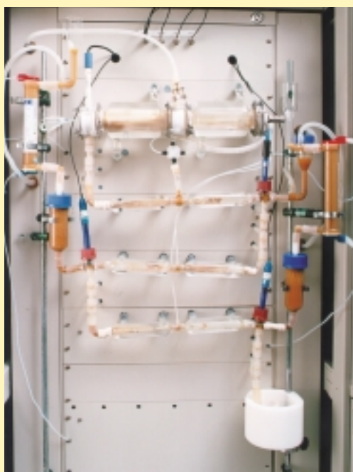
Fig. 5 Picture of the TNO dynamic model of the stomach and small intestine (TIM-1)
